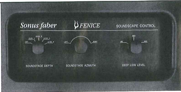
ABOVE: Sound Field Shaping is adjusted by – in addition to rear sub-speaker orientation – twin rotary controls labelled soundstage depth and soundstage azimuth, the former adjusting output level. A third control adjusts subwoofer level
